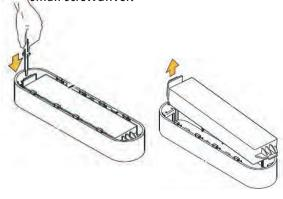
2. Install 2AAA alkaline batteries (included).
